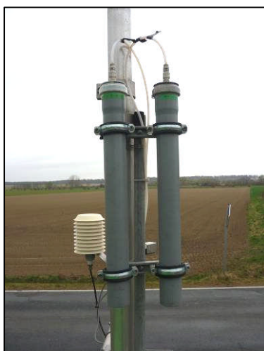
Abb. 6: Denuderrohre in HT-Rohren (GAA-HI)
